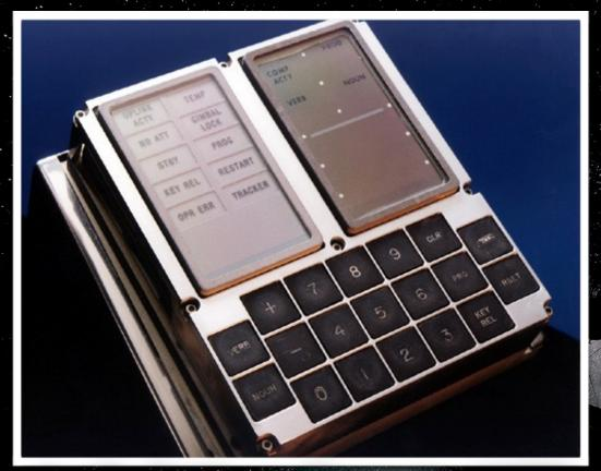
The computer used an operating system which allowed astronauts to type in nouns and verbs that controlled their spaceship.
